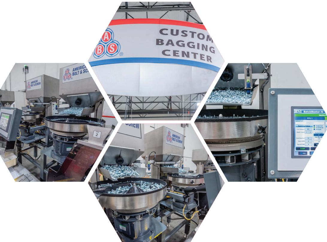
Batchmaster Counters are the only counters that utilize patented dual view scanners that provide the highest accuracy count possible. Out of tolerance parts are rejected prior to entering a package. The latest Batchmaster IV counter is an accurate high speed counting system that detects and rejects parts one-third smaller or larger than a target part thereby separating the good parts from the bad.
